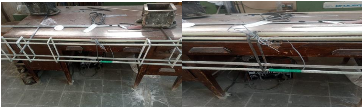
Figure (2): Position of reinforcement strain gauges.
